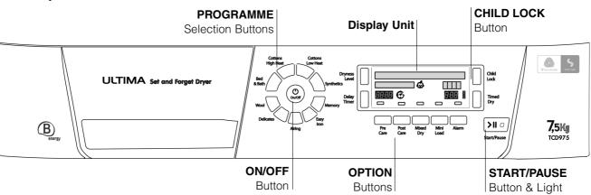
The **ON/OFF** button/light 0: If the dryer is running and this button is pressed, the dryer is turned off. Press again, the dryer restarts.
